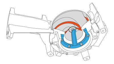
In wastewater treatment plants, more often than not, a **high amount solid waste**, even of large size, tends to build up inside the collection tanks, potentially **blocking the impeller** and **clogging up the pipes** making the lifting station almost ineffective.
